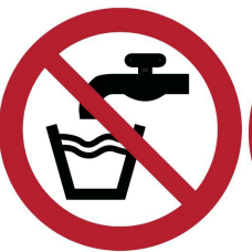
P005 - Eau non potable
